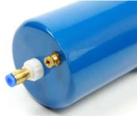
Manual drain (SD02) valve is fitted as standard on filter MS040 (¾") and larger for rapid depressurisation and autodrain function check.
